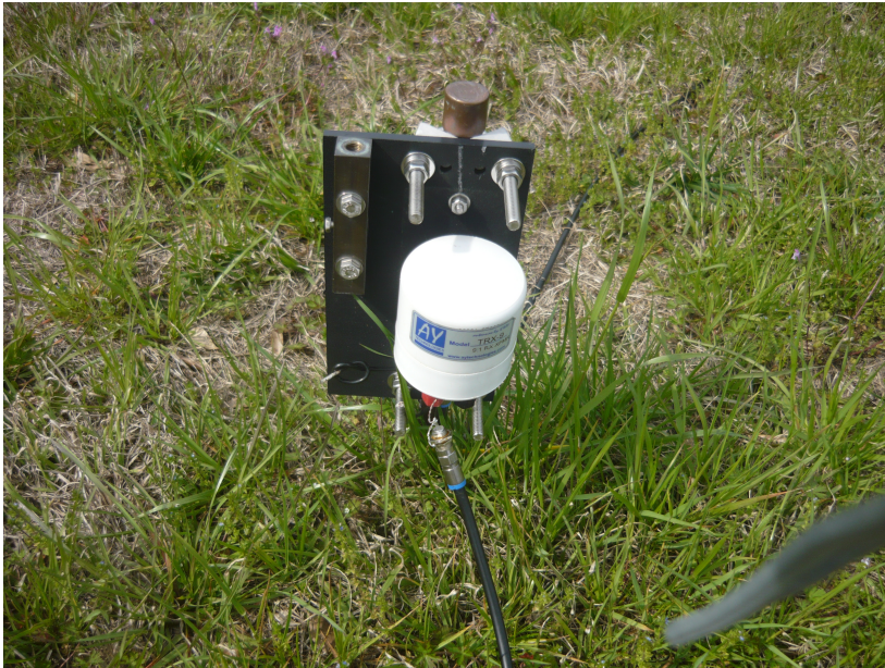
Feedpoint K9AY Loop Transformer
