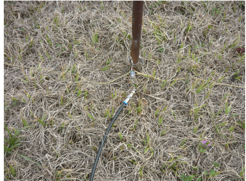
BOG Termination 270 Ohms + 2 Radials
